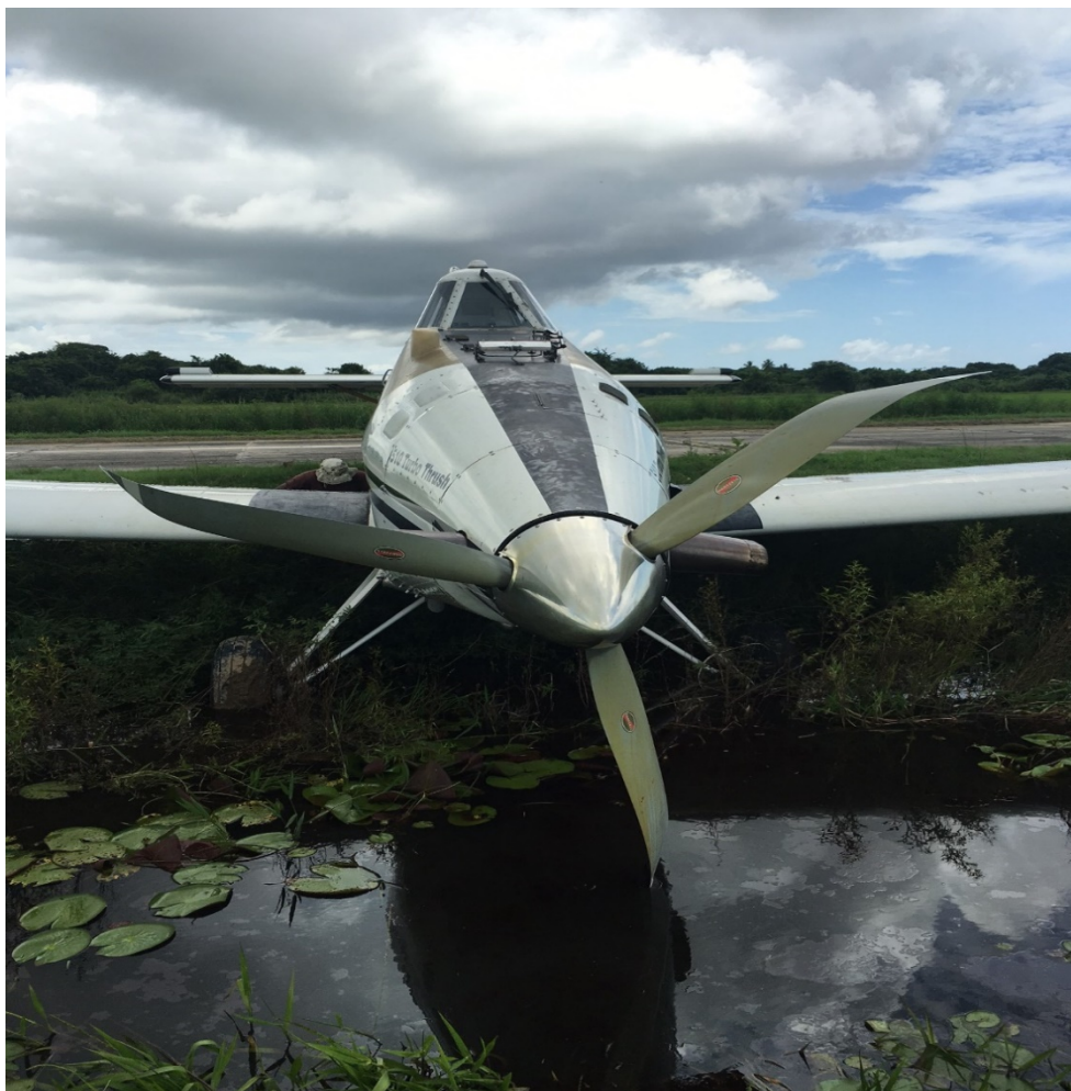
Picture showing final position of aircraft and damage to propellers
